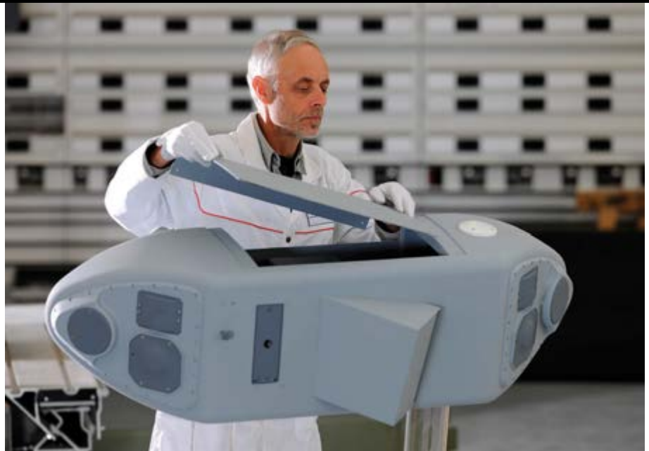
The ISSYS POD system for helicopters packages Saab’s Compact Integrated DAS into a pair of RUAG-developed pod enclosures. (Photo: RUAG)
