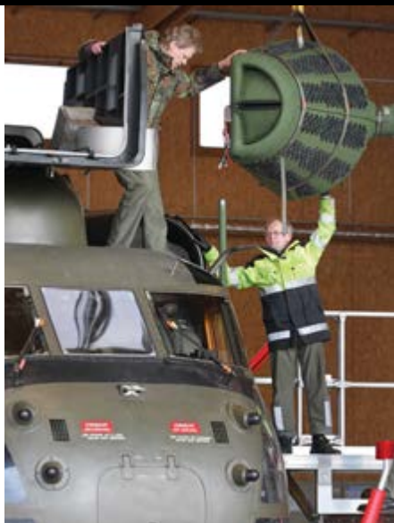
Engine air particle separators for the German CH-53 fleet originate from the US 'boneyard' at Davis-Monthan AFB. (Photo: Bundeswehr)
